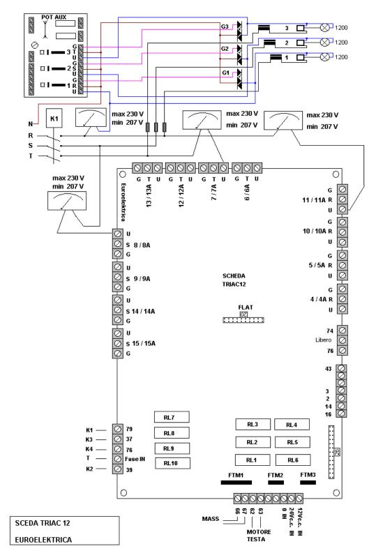
TRIAC Board Voltage Measurements for Lamp Intensity Adjustment
