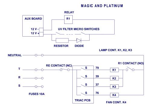
CONTROL CIRCUIT FOR LAMP AND FAN CONTACTORS
